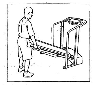
2. Move your right hand to the position shown and hold the treadmill firmly. Raise the treadmill until the storage latch closes over the catch. Make sure that the storage latch is fully engaged over the catch.
